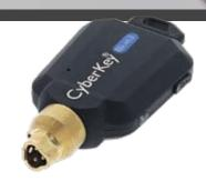
The CyberKey Blue 3 is an electronic key used to operate CyberLock cylinders and FlashLock access points. It has memory that contains encrypted access codes, a list of locks it may access, schedules of authorized dates and times it may access locks, and a begin-end date range during which the key will operate. The battery from a CyberKey energizes the electronics within a CyberLock cylinder.
