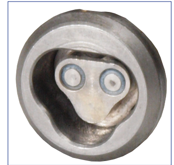
Figure 1 – Dirty Lock Face
