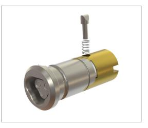
Figure 3: Remove, Clean Pin and Spring
